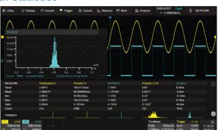
Parameter measurements include 4 categories: Vertical, Horizontal, Miscellaneous and Channel Delay providing over 50 different types of measurements.
