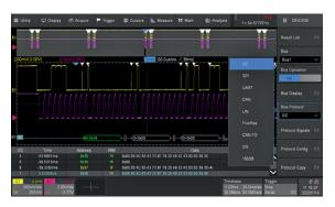
Trigger and decode up to 2 common embedded and automotive serial buses, I<sup>2</sup>C, SPI, UART, LIN, CAN, CAN FD, FlexRay, I<sup>2</sup>S, MIL-STD-1553B, SENT and Manchester. Protocol information can be quickly and intuitively displayed, time aligned with the waveform and in table format.
