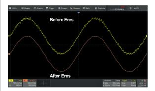
Enhanced Resolution (ERES) function reveals hidden waveform detail by using a linear average filter to reduce waveform noise on single acquisition waveforms, where regular averaging will not work. The ERES acquisition mode is hardware based, allowing waveforms to be captured at a faster rate.
